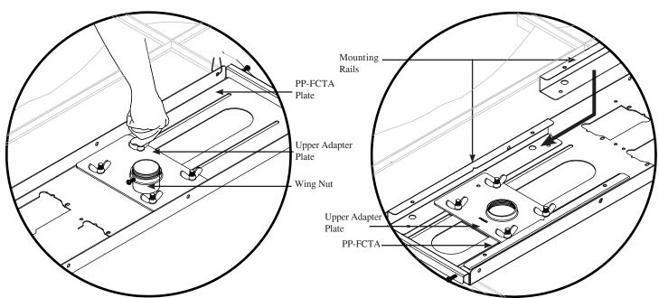
**Step 1.** Loosen the wing nuts (do not remove) on the upper adapter plate.
